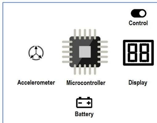
Figure 1. Pedometer Block Diagram.
